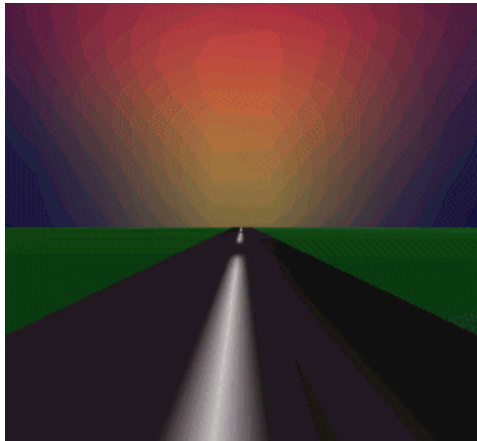
Figure 6.8 Sphere background geometry. A texture image was applied to the sphere and normal vectors generated such that the texture is visible when viewed from within the sphere
