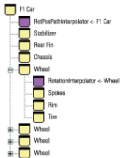
Figure 11.1 A scenegraph branch for the Formula 1 racing car. The branch contains five Behaviors , the first ( RotPosPathInterpolator ) to replay the car through a recorded trajectory, and four RotationInterpolator Behaviors —one to rotate each wheel
